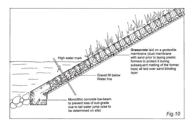
With its traffic bearing capability, GRASSCRETE can be specified as a 'total' armour layer to reservoir bunds with crest access for heavy vehicles being accommodated.
