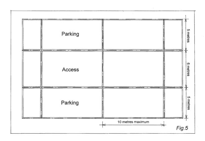
In addition to the general parking provided under fig.5, further delineation can be provided by transverse strips of concrete formed by the omission of a 200mm part segment of a former. This can be either to the full width of a bay or in a truncated 'tee' format (see fig.6).
